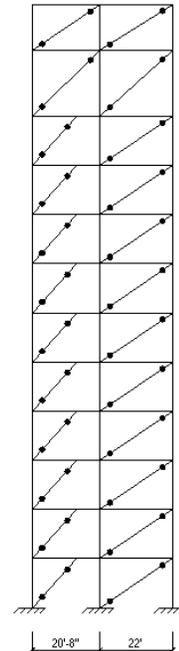
Figure 3: Braced Frames
