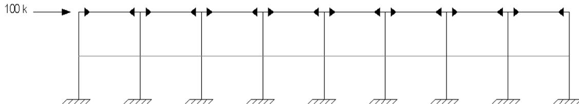
**Figure 14: Frame Loading for Relative Stiffness**
