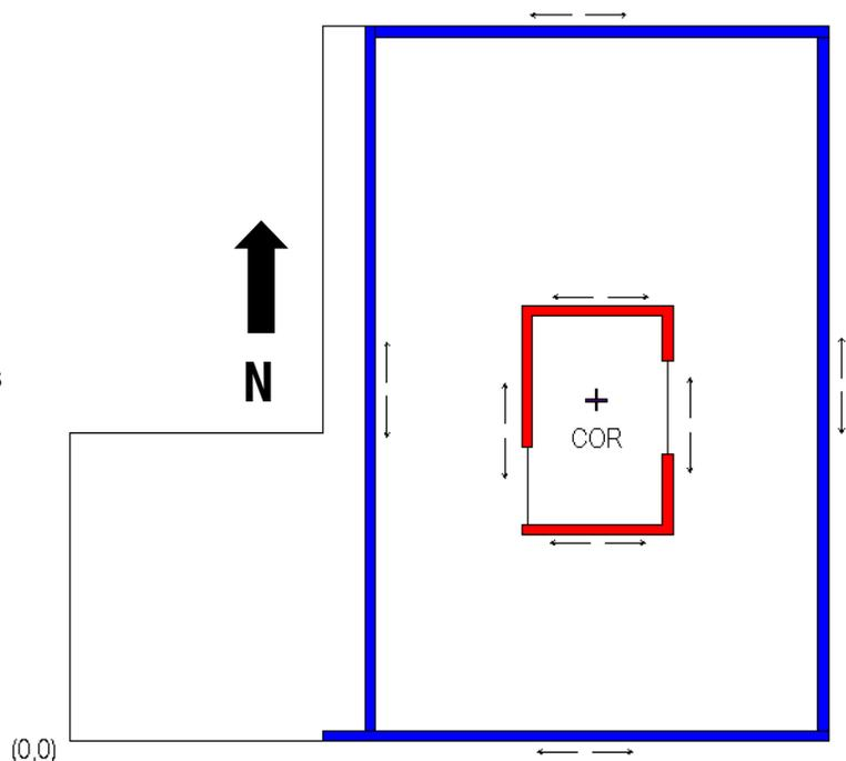
Figure 18: Level 1 Floor Plan with COR shown
